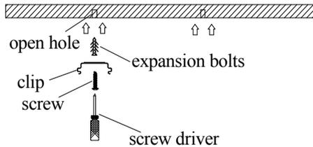
C. fasten the luminaire onto the clips.
