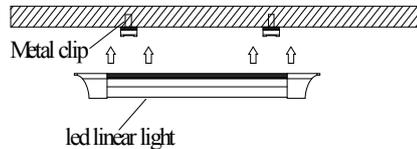
D. Adjust the position of the fixture
